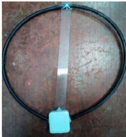
**Figure 3** Main Loop with Capacitors' Box
