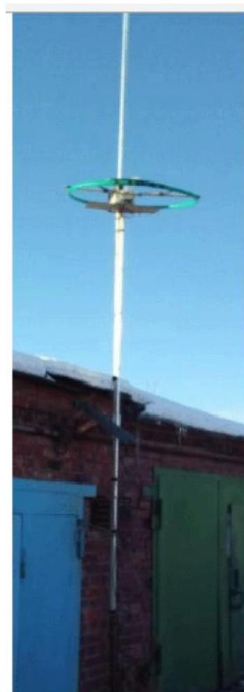
**Figure 4** Installed UA6AGW Antenna with Vertical Radiators in tested position
