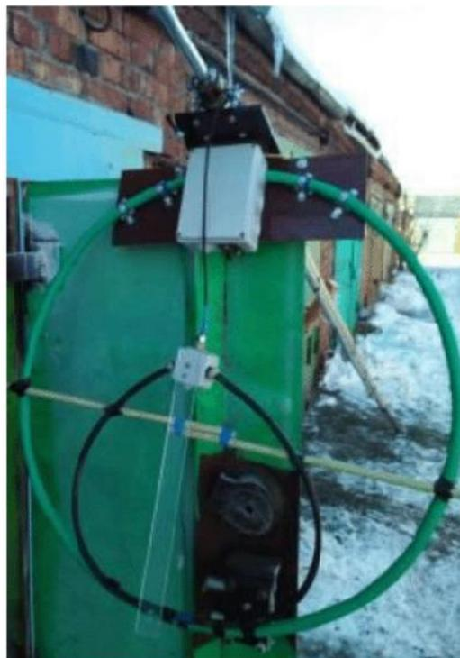
Figure 5 Coupling Loop at the Main Loop
