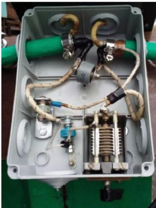
**Figure 2** Capacitors Inside of Waterproof Electrical Box
